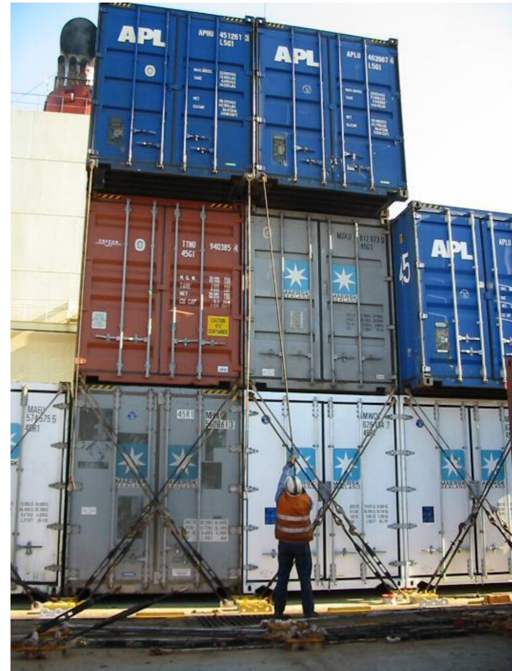
Figure 8. Turnbuckles used to secure containers on board a ship ( en.m.wikipedia.org/ ).
