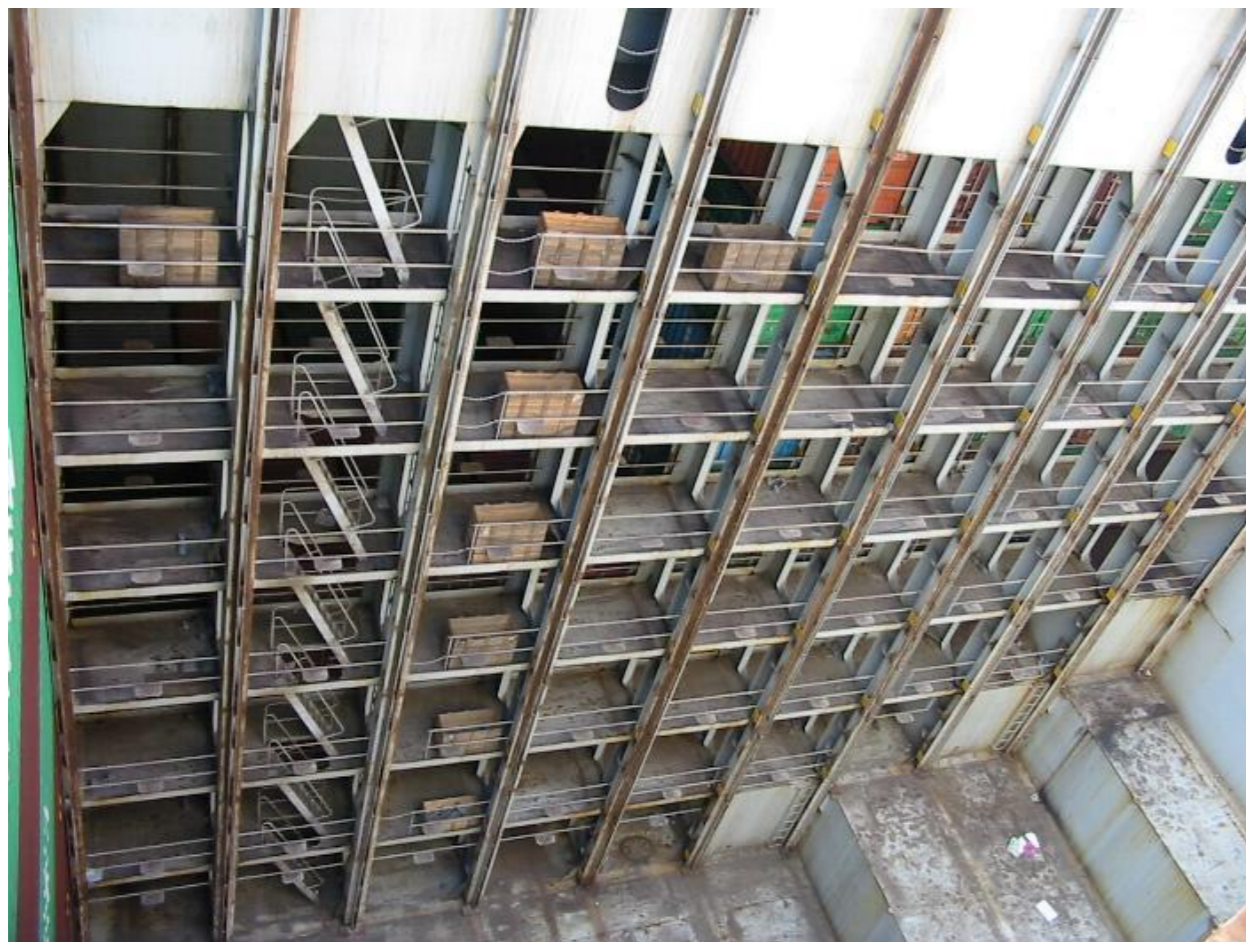
Figure 7. Internal web frames of a ship give it additional strength ( http://www.portpictures.nl ).
